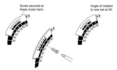
Figure-6 Securing the AM-689 Rotation Limiter.
