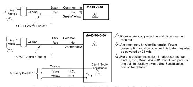
Figure-3 Typical Wiring Diagram for 24 Vac Basic and Single Auxiliary Switch Models.
