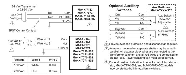
MX40-707X-502 and MX40-715X-502 units manufactured prior to the date code 0141 (October 6, 2001) used the following color coding for the auxiliary switches:
