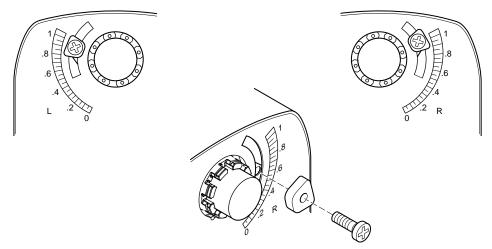
Figure-5 Adjusting Stop Block for Limited Rotation.
