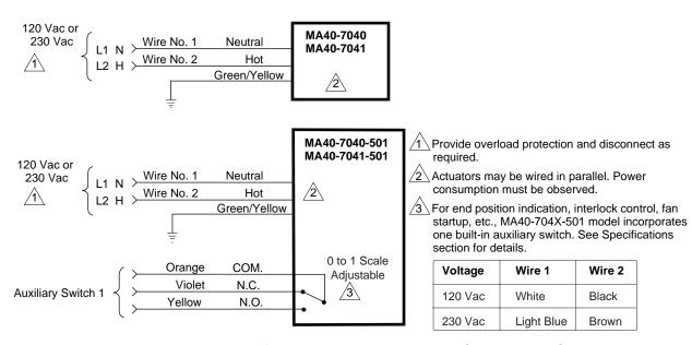
Figure-2 Typical Wiring Diagram for 120 Vac or 230 Vac Basic and Single Auxiliary Switch Models.
